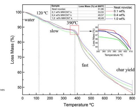
**FIGURE 5** Thermogravimetric analysis curves for neat novolac resin and the nanocomposites at  $\beta = 10^{\circ}$ C/min in N2 [Colour figure can be viewed at wileyonlinelibrary.com]
