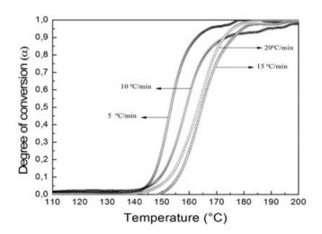
**FIGURE 2** Degree of conversion as a function of the reaction temperature at different heating rates for neat novolac
