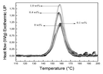
**FIGURE 3** Heat flow as a function of temperature for neat novolac and novolac/o-MWCNTs nanocomposites at a heating rate of  $\beta = 10^{\circ}$ C/min
