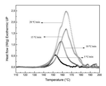
**FIGURE 1** Heat flow as a function of temperature for the novolac resin with 7 wt% HMTA catalyst at different heating rates  $\beta$
