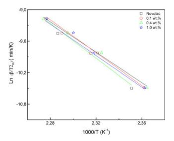
**FIGURE 4** Isoconversional plot for neat novolac resin and their nanocomposites [Colour figure can be viewed at wileyonlinelibrary. com]
