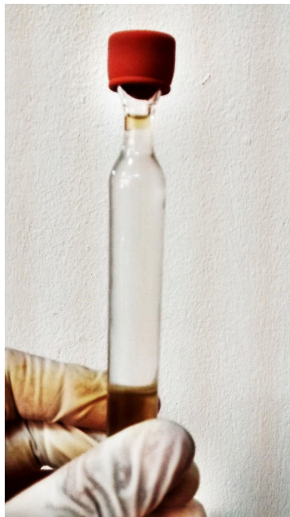
Figure 1. Photograph of the separated RTIL-water phases after centrifugation within the narrow-neck glass tube.
