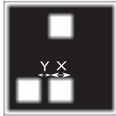
Figure 1. Proposed information container for a single character ‘C’. X is the block size and Y the block separation.
