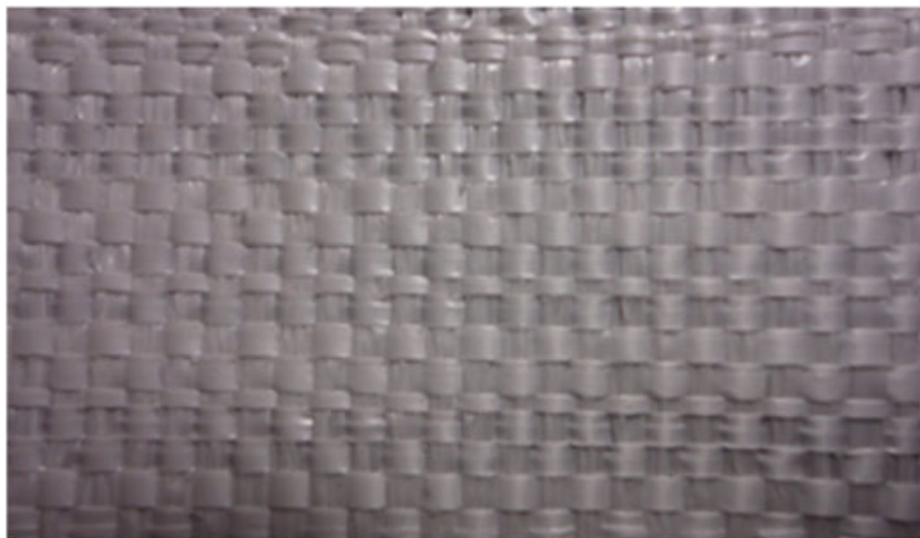
FIGURE 2 Commercial woven PP fabric used as reinforcement [Colour figure can be viewed at wileyonlinelibrary.com ]
