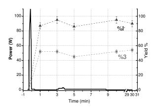
Figure 1. Reactions under N<sub>2</sub> atmosphere heated by microwave irradiation (150 W max) for 30, 10, 5, 3 and 1 min after irradiation. Acetophenone (1.5 mmol), tBuOK (2.5 mmol) and PhI (0.5 mmol) in 2 mL of DMSO. In light 50 in dark gray triangule % I, determined potentiometrically using a Ag/Ag(I) electrode. Typical power applied to these experiments from the CEM discover Microwave reactor in solid black line.
