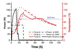
Figure 2: Comparison of temperature (red) and power (black) profiles for dynamic mode heating (solid) and experiments at fixed power at 50W (dash) and 100W (dots).
