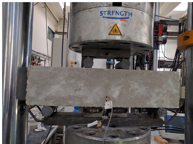
Fig. 8. Experimental set-up of the four-point bending test.
