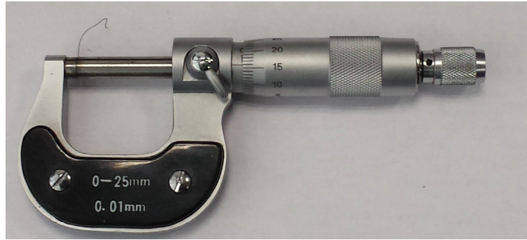
Fig. 2. Characterization of fibers: micrometer for the diameter measurements.
