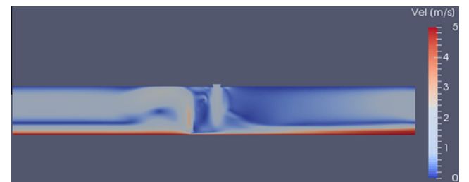
Fig. 5b. Simulated speeds values involved in the P 1 point. Values for G = 4 mm and Z = 0.7 mm.
