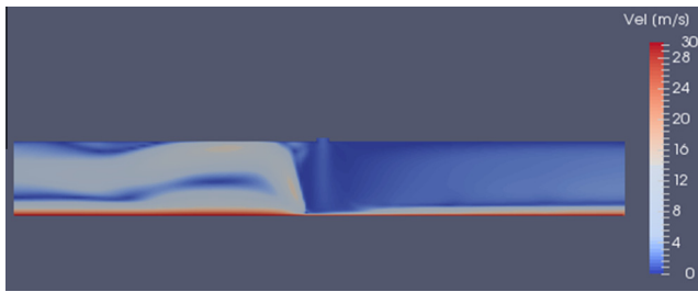
Fig. 7b. Simulated speeds values involved in the P_3 point. Values for G = 4 mm and Z = 0.7 mm.
