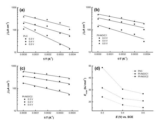
Fig. 6. Arrhenius plots of the overall ethanol oxidation rate in 1 M CH<sub>3</sub>CH<sub>2</sub>OH/0.5 M H<sub>2</sub>SO<sub>4</sub> solution for Pt/C (a), Pt–NiO/C1 and Pt–NiO/C2 (c) at different potentials. (d) Apparent activation energies for the overall EOR at different potentials. Data taken from steady-state reaction currents.
