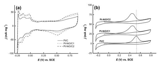
Fig. 3. (a) Steady cyclic voltammograms of the different carbon supported Cu@Pt-Ru core-shell catalysts in 0.5 M H<sub>2</sub>SO<sub>4</sub> at room temperature and  $\nu = 50$  mV s<sup>-1</sup>. (b) Voltammetric curves for adsorbed CO stripping on the Pt/C, Pt-NiO/C1 and Pt-NiO/C2 electrocatalysts in 0.1 M H<sub>2</sub>SO<sub>4</sub> at 10 mV s<sup>-1</sup>.
