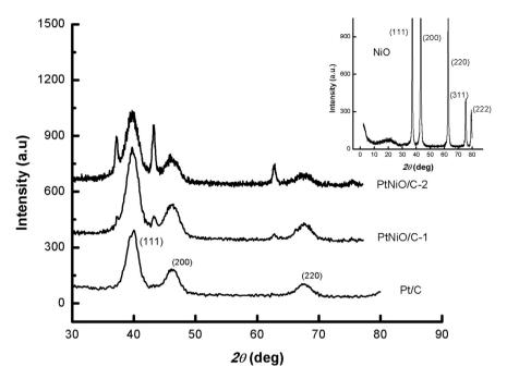
Fig. 1. XRD patterns of Pt/C and Pt-NiO/C catalysts. Inset: XRD pattern of the pure NiO sample.
