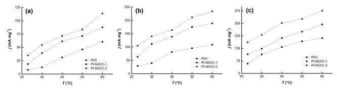
Fig. 5. Steady-state current densities during constant potential ethanol oxidation (1 M CH<sub>3</sub>CH<sub>2</sub>OH/0.5 M H<sub>2</sub>SO<sub>4</sub>) at different potentials and temperatures. (a) 0.3 V, (b) 0.4 V and (c) 0.5 V.
