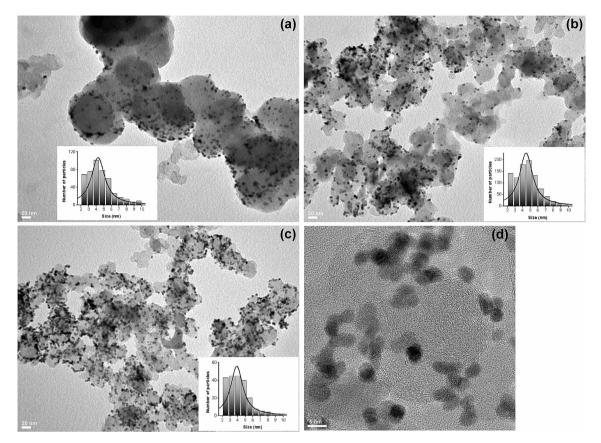
Fig. 2. TEM images and particle size distribution (inset) of the as-prepared electrocatalysts used in this work: (a) Pt/C, (b) Pt-NiO/C1 and (c) Pt-NiO/C2. (d) HRTEM image of Pt-NiO/C2 catalyst.
