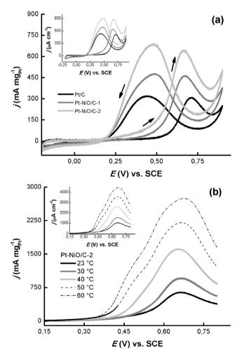
**Fig. 4.** (a) Steady cyclic voltammograms (thirtieth cycle) for the different electrodes in 1 M CH<sub>3</sub>CH<sub>2</sub>OH/0.5 M H<sub>2</sub>SO<sub>4</sub> at room temperature. (b) Linear sweep voltammograms for ethanol oxidation on Pt–NiO/C2 electrode at various temperatures. The sweep rate was 50 mV s<sup>-1</sup> and the arrows indicate the scan direction.
