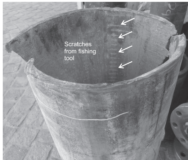
Fig. 6. Lower tract of failed casing.
