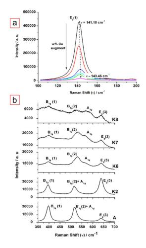
**Figure 8.** Variation of anatase Raman vibration peaks intensity versus  $Ce(Val)_3/TTIP$  molar ratio: (a)  $E_g(1)$  and (b)  $B_{1g}(1)$ ,  $B_{1g}(2)$  and  $A_{1g}$  Raman active modes.
