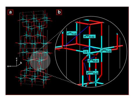
Figure 5. Schematic representation of (a) anatase crystalline unit cell and (b) Ti-O and O-O distances in a regular tetrahedral anatase crystal.
