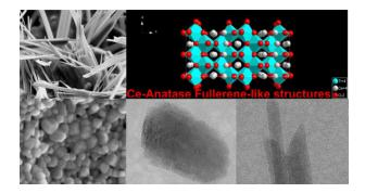
The presence of Ce atoms has a clear influence in the  $TiO_2$  substrate morphology, distorting anatase crystal lattice, inducing the formation of fullerene-like structures and increasing its oxygen storage capacity. It was demonstrated that such special effects can be exploited to modulate the fibroblast proliferation.
