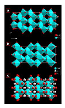
**Figure 6.** Schematic representation of **(a)** regular anatase crystal, **(b)** K2 sample without considering the incorporation of Ce atom to the anatase structure and **(c)** K2 sample incorporating the Ce atom to the anatase structure.
