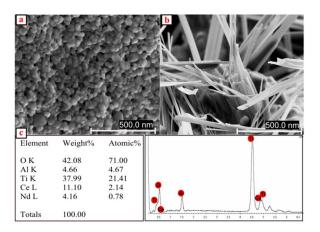
**Figure 1.** Scanning electron microscopy (SEM) microphotographs of **(a)** K2 and **(b)** K8 materials after annealing at 650°C during 6h in an air flux. **(c)** Energy-dispersive X-ray (EDX) of K8 sample.
