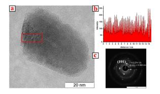
Figure 3. (a) H-TEM of 6.0 × 10<sup>-3</sup> Ce(Val)<sub>3</sub>/ TTIP molar ratio fullerene-like particles (sample K4).
