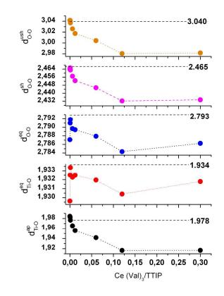
**Figure 7.**  $d_{Ti-O}^{eq}$ ,  $d_{O-O}^{ap}$ ,  $d_{O-O}^{eq}$ ,  $d_{O-O}^{sh}$ ,  $d_{O-O}^{ush}$  distances variation versus Ce(Val)<sub>3</sub>/ TTIP molar ratio. Computed considering u = 0.208 (regular anatase crystal)
