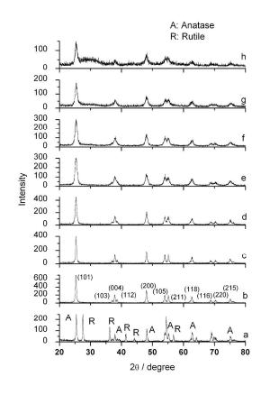
**Figure 4.** X-ray diffraction pattern of different synthesized CeO<sub>2</sub>-TiO<sub>2</sub> samples: **(a)** K1, **(b)** K2, **(c)** K3, **(d)** K4, **(e)** K5, **(f)** K6, **(g)** K7 and **(h)** K8.
