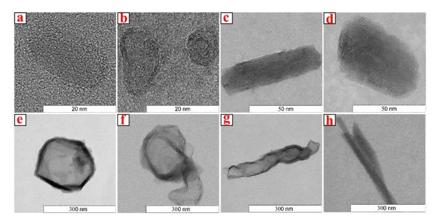
**Figure 2.** H-TEM images of different synthesized CeO<sub>2</sub>-TiO<sub>2</sub> samples: (a) K1, (b) K2, (c) K3, (d) K4, (e) K5, (f) K6, (g) K7 and (h) K8.
