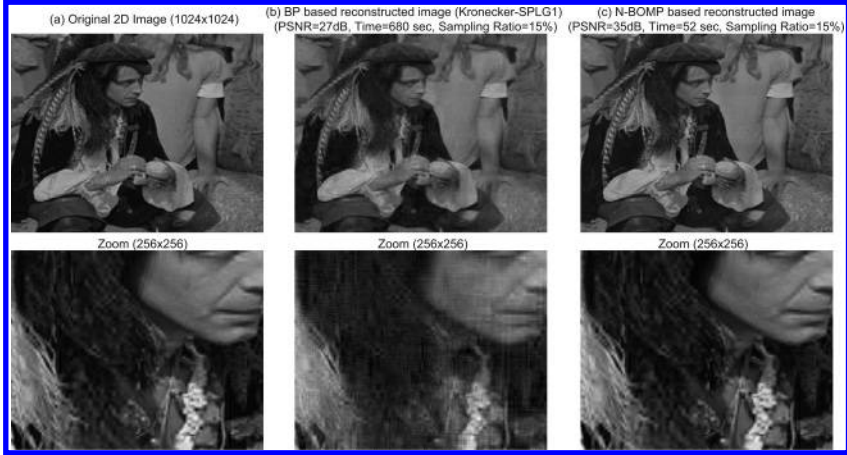
Figure 8: Compressive imaging example of a 1-megapixel image using 397^2 samples (i.e., 15% of the original image size). (a) Original image approximated with 99,078 wavelet coefficients contained in a 294 \times 337 2D block. (b) Kronecker-SPLG1 (Rivenson & Stern, 2009a) reconstruction. (c) N-BOMP reconstruction.
