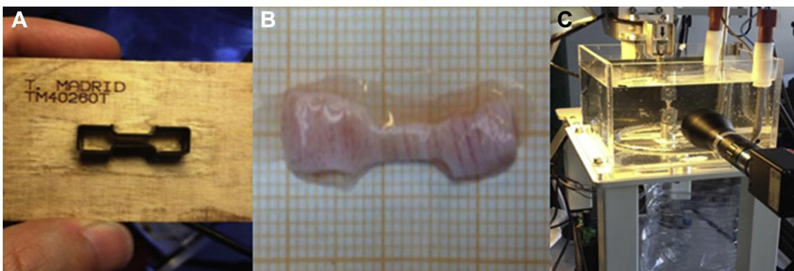
**Fig. 2 – (A) A 10-mm dog-bone punch. (B) Dog bone tissue sample. (C) Tensile test apparatus. (Color version of figure is available online.)**
