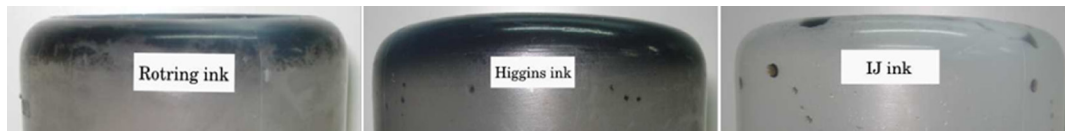
Figure 3. Receptacles of ink dilutions after 60 days, after ultrasonic mixing procedure (the large spots in the IJ container are droplets of the dilution).
