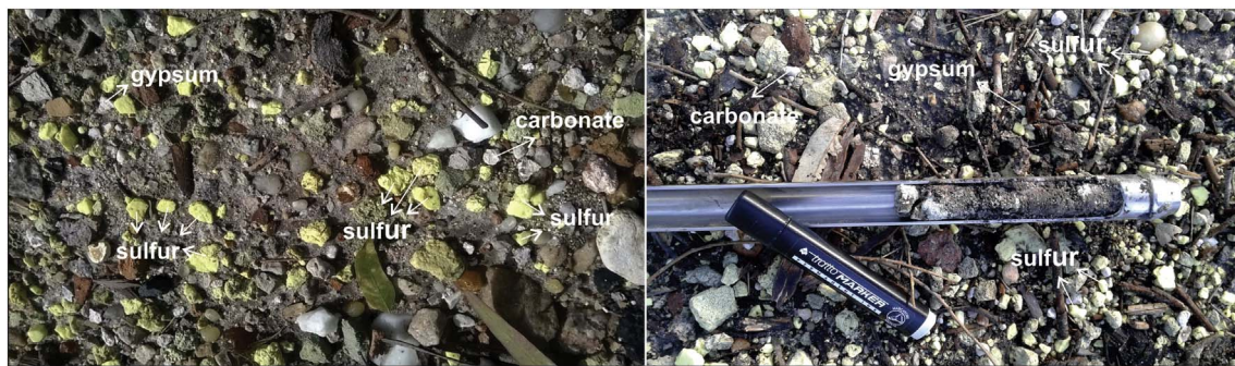
Fig. 7. Clastic grains of sulfur, gypsum and carbonate in topsoils affected by wastes of a sulfuric acid plant.
