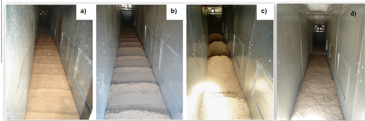
Fig. 1. View of the soil surface conditions produced by different tillage tools: (a) disk tandem (DT), (b) drill-hoe (DH), (c) lister-bedder (LB) and (d) flat surface (FS).
