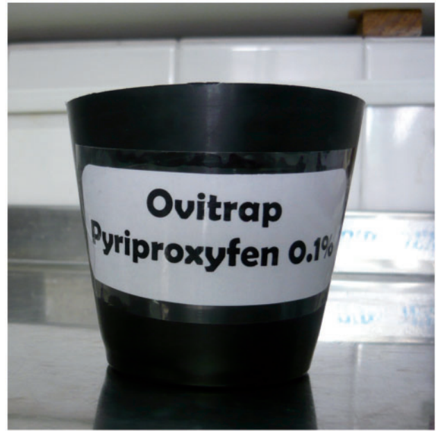
Fig. 1. Ovitrap prototype made of LDPE with pyriproxyfen 0.1% w/w.
