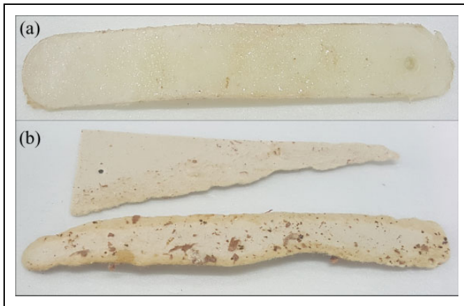
Figure 5. (a) AMZ/EVA strip and (b) commercial strips; after their use in hives during 28 days of varroasis treatment. AMZ: amitraz; EVA: ethylene-vinyl acetate.
