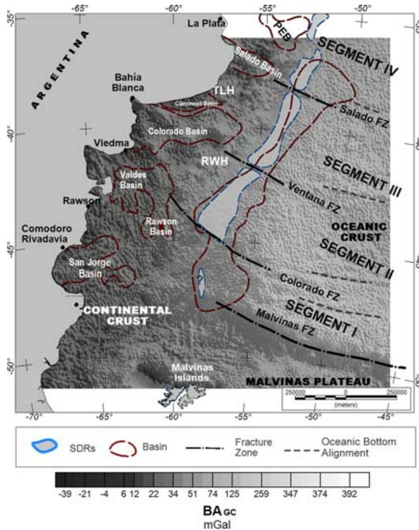
**Figure 2.** Bouguer anomalies with geological correction. The Bouguer anomalies were calculated and corrected by geological correction.  $BA_{GC}$  map shows positive values which realize make clear the crustal thinning, as well as, under both Colorado and Salado basins on the continental shelf, and on deep Argentina basin. For references see Fig. 1(A).
