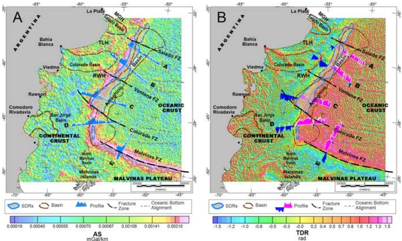
**Figure 3.** Enhancement techniques applied to the Argentine continental margin. (A) Analytic signal (AS) and (B) tilt angle (TDR) maps are shown. In both maps, five transverse rotated profiles of the respective applied techniques, major Fracture Zones and the most significant sedimentary basins according to their gravitational weight are shown. For references see Fig. 1(A).
