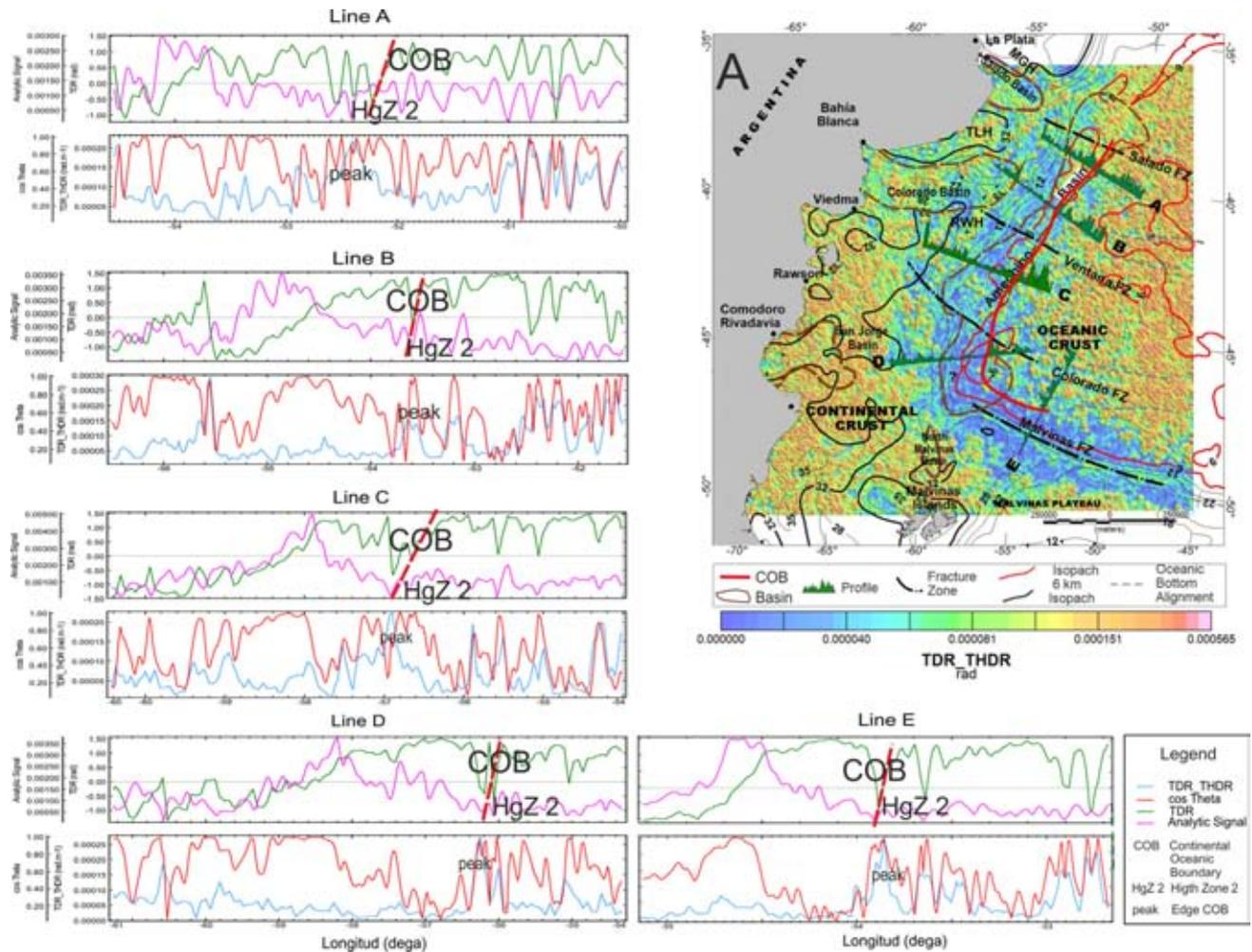
**Figure 8.** (A) Map of the location of the COB (red line) and the isopach crust–mantle discontinuity on the grid of the total horizontal derivative of the tilt angle. Lines A, B, C, D and E: Transverse profiles of the analytic signal, Theta map, tilt angle and total horizontal derivative of tilt. COB interpretation is indicated in lines A, B, C, D and E with the red line. The location of lines A, B, C, D and E is shown in panel (A).
