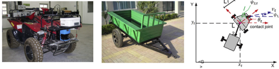
Fig. 1 – Service unit used in this work, its passive trailer and its corresponding kinematic model. Left shows a bicycle-like robot, middle is the trailer used during the harvesting experiments, right shows a schematic of the kinematic model of the service unit with a trailer.
