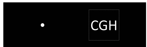
Fig. 3. Schematic of the mask composed by a pinhole and a binarized amplitude hologram.
