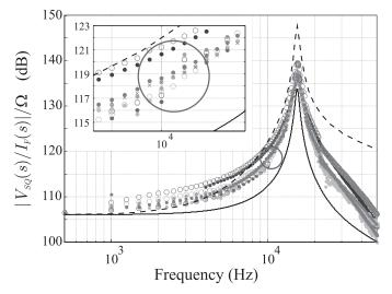
Fig. 5. Absolute value of the frequency response of the initial model (black dashed curve), identified model (black solid curve), and the experimental data measured with a lock-in amplifier. Different colored lines distinguish the different measurement days.
