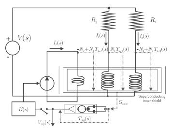
Fig. 2. Schematic of the two-terminal CCC. The notation for the transfer functions from the origin to the end of the blue-dotted arrows is indicated. In the feedback loop, a switch is included to indicate where the loop is opened.
