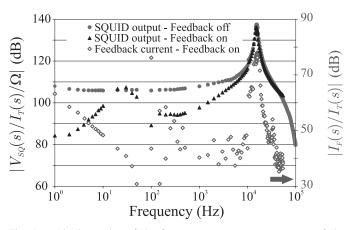
Fig. 1. Absolute value of the frequency response measurements of the SQUID voltage from a test current  $I_T(s)$  in a single-turn winding, with integral feedback OFF (red circle) and ON (black triangle). The response of the feedback current from the same input in closed loop is shown in the secondary axis (blue diamond).
