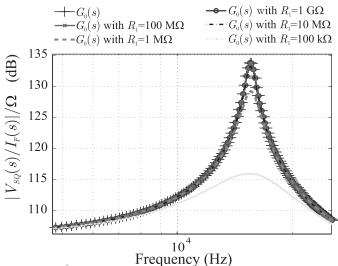
Fig. 4. Simulation of  $G_0(s)$  (5) with six values of  $R_1$ . The transfer function for large value of resistance presents low deviations.
