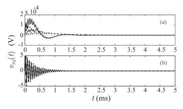
Fig. 9. (a) Step and (b) impulse simulated responses of the closed-loop system for the identified model (black dashed line) and the worst case model (blue solid line). The excitation amplitudes were 0.1 pA in the primary winding in both cases.
