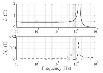
Fig. 3. Measurement results of  $L_1$  and  $M_{1F}$ , in the top and bottom figures, respectively. The values at cryogenic (red star) and ambient (red circle) temperatures are shown. The simulations for the self-inductance at 4.2 K (blue solid line) and the mutual inductance at 300 K (blue dashed line) are also presented.
