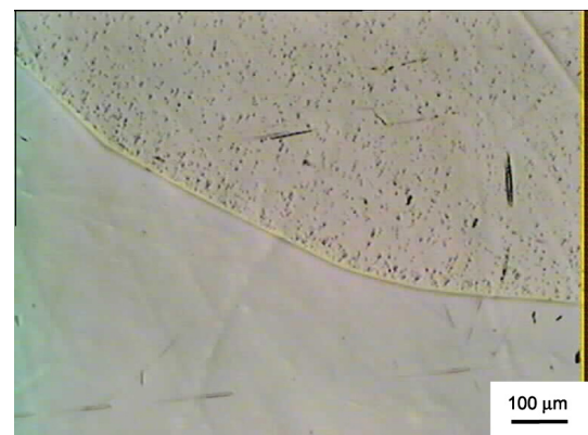
Fig. 1. Optical micrograph (5 \times ) corresponding to a typical \alpha -Zr sample after growth and stabilization annealing. A few large grain sizes were obtained.
