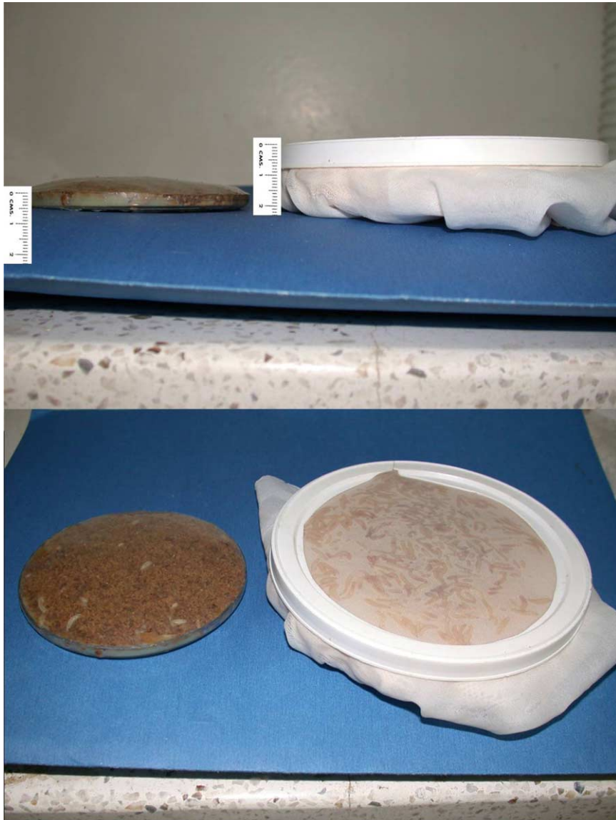
Figure 3. Modified Petri dish (M-PD) oviposition unit used to rear U. anastrephae , the parasitoid species with the shortest ovipositor (left). For comparative purposes (i.e. distinguish differences in thickness of oviposition unit), a 'sandwich-type oviposition device' is also shown (right).
