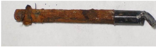
Fig. 6. Optical microscope image of a steel bar after the extraction from the mortar specimen (specimen type A, w/c 0.6, i_{app} = 750 \mu\text{A}/\text{cm}^2 , t = 6 days).
