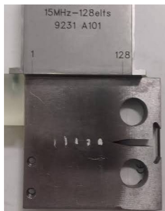
Figure 6 – Picture of the experimental set-up. Compact Tension sample (according ASTM E647 – 13ae1) along with array transducer of 128 elements operating at 15 MHz.
