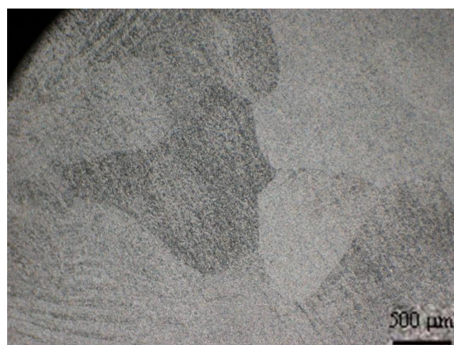
Figure 1: Optical micrography (5x) corresponding to a typical Nb sample.
