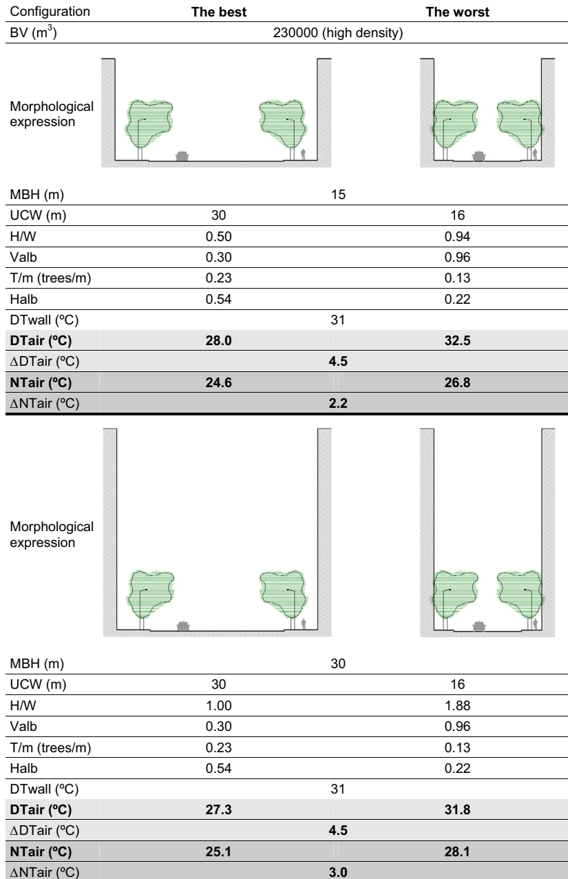
Fig. 10. The best and the worst cross-section's configuration in high building density according to thermal behavior for day and nighttime.
