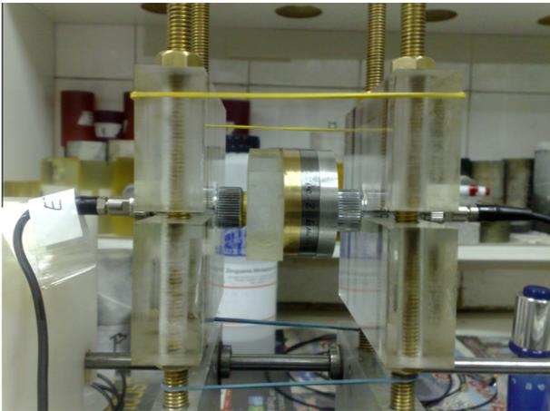
Fig. 12. Configuration I with transducers in contact with the sample.
