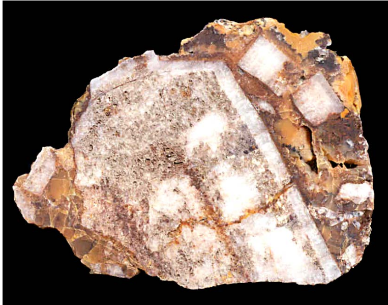
FIG. 5. The feldspar sample from the San Luis II pegmatite, cut in the [010] zone at an oblique angle to c ; the perthitic microcline (white, mottled, medium grey where altered) in central parts, overgrown by nonperthitic microcline (pale grey to off-white). Rusty-colored "chalcedony" and opal fill interstices between the main crystal and smaller ones (top right). The sample is 10 cm wide.
