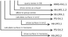
Fig. 11. Service interaction to implement the function calculate zone surface in different measures.
