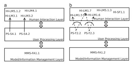
Fig. 10. Set of services within the architecture to implement two generic functionalities. (a) Calculate zone surface in different measures and (b) query station attributes.
