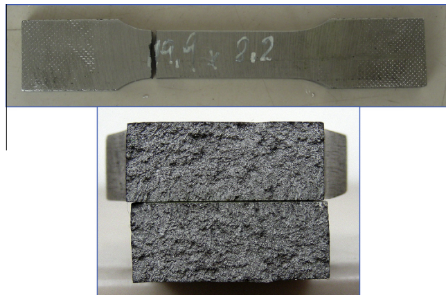
Fig. 8. Tensile test specimen (longitudinal) and fracture surface.
