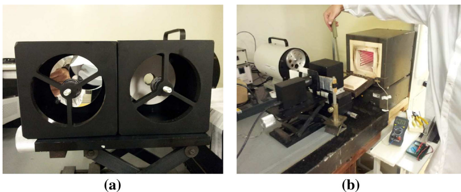
Fig. 4 a Two telescopes identical to those used in SOLAR-T were built to measure the losses of a rough surface compared to a polished mirror. b A furnace radiator on the right, large enough to cover the whole telescope aperture was heated at a fixed high temperature. The output using the polished and the roughened telescopes were made alternatively, using a 2 THz band-pass filter. The transmission by the rough surface mirror was about 0.9 compared to the polished mirror
