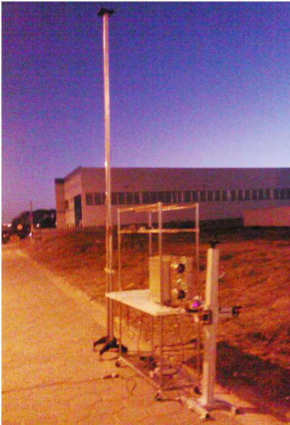
Fig. 12 Realistic operational tests performed with SOLAR-T “on-board” setup, with hot source in front of telescopes, coupled to Iridium antenna at the top of the mast. Results are shown in Fig. 13
