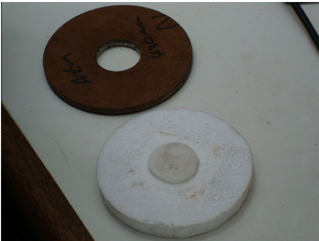
Fig. 7. Polystyrene blast platform.
