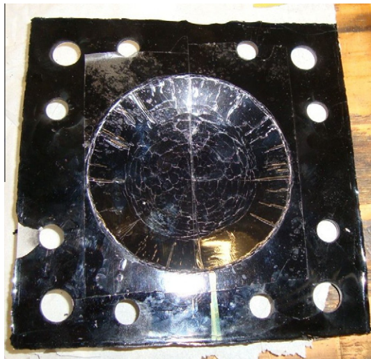
Fig. 12. Fracture pattern of epoxy/CNT core.
