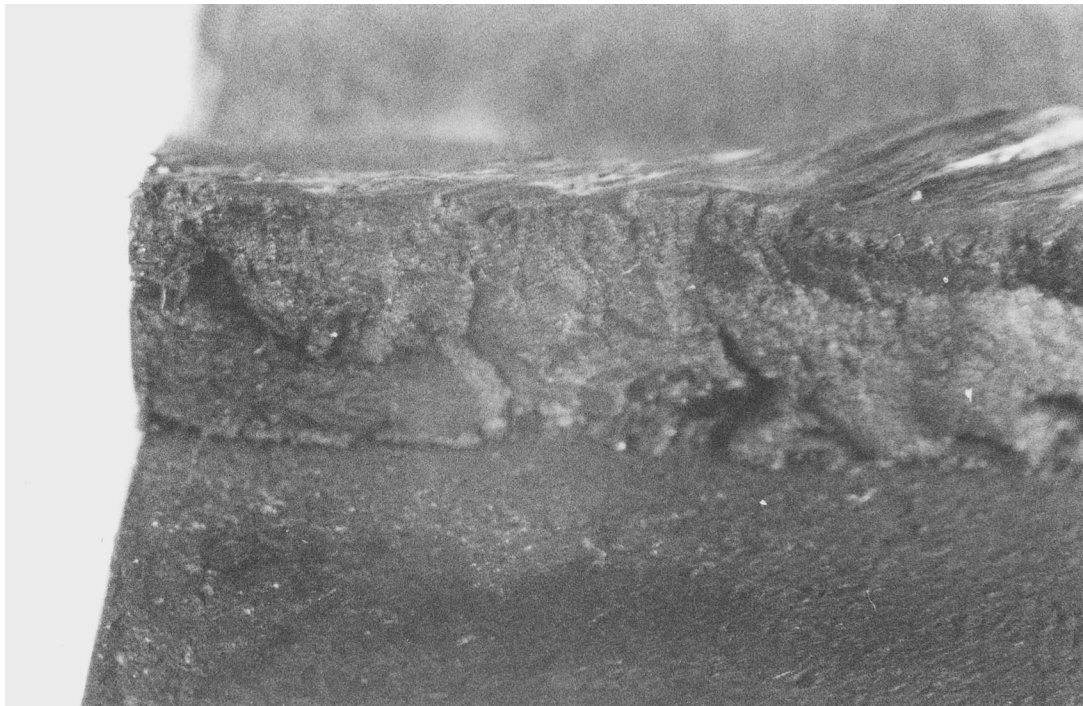
Fig. 9. Weld-side fracture surface, showing signs of lack of fusion.
