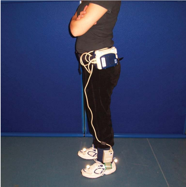
Figure 1. Equipment used for data collection in one of the subjects who participated in this study. The subjects were fitted with markers on heels and toes, and with insoles inside the shoes and a portable datalogger on their waist for capturing and storage of pressure measurement data.
