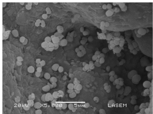
Fig. 2. SEM micrograph of a scaffold 45S5.2B exposed in vitro to S. aureus (ATCC 29213) for 24 h.
