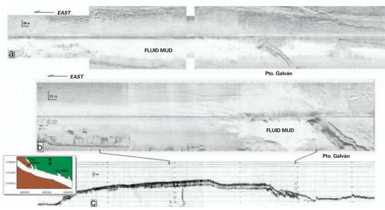
Figure 3. Side scan sonar records from the Canal Principal before and after the dredging showing the presence of mud fluid layers at the bottom of the channel.
