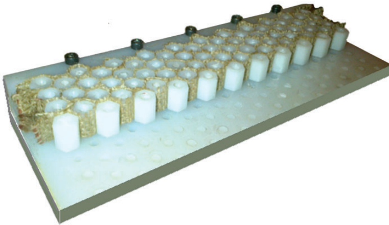
Figure 3. Plastic mold used for manufacturing the honeycombs.
