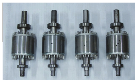
Fig. B.1. Induction motor rotors: healthy, one, two and three broken bars.
