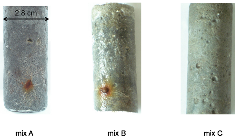
Fig. 5. Images of the mortars with rebars after 365 days of immersion.
