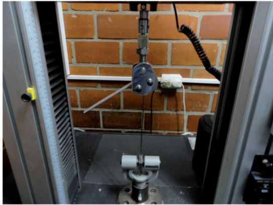
Figure 9. Device used to measure the degree of tack of the prepregs.
