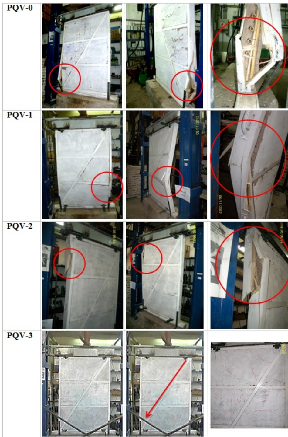
Figure 8. Sequence of wattle and daub walls to compression load tests
