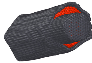
Fig. 11. Illustration of how two open ended misaligned different diameter iron filled CNTs stick together at the end (stage h of Fig. 10) of the soldering process shown in detail in Fig. 10.
