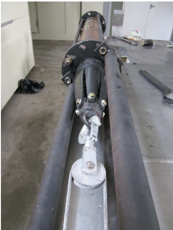
Fig. 2. Liner insertion system for buckling collapse tests.
