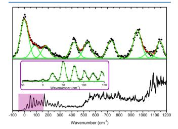
**Figure 2.** Low-energy part of the spectra of the  $C_2H^+$  (upper panel) and  $C_2Ag^+$  (lower) complexes. In the lower panel, the inset shows an amplification with better resolution of the first 150 cm<sup>-1</sup> of the spectrum of the  $C_2Ag^+$  complex, in which a low vibrational frequency progression composed of narrow bands is observed. The vibrational bands were fitted to Voigt profiles.
