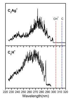
**Figure 1.** Photofragmentation spectra of the  $C_2Ag^+$  and  $C_2H^+$  complexes in the whole spectral range analyzed in this work (225–320 nm). Vertical dashed lines show the wavelengths of the origins of the electronic transition of the individual components of both complexes,  $C^{39}$  and  $CH^+$ .  $^{30}$ The electronic transition wavelengths of Ag (328.2 nm) $^{40}$  and Ag $^+$  (110.7, 111.2, and 119.6 nm) $^{41,42}$  fall out of scale.
