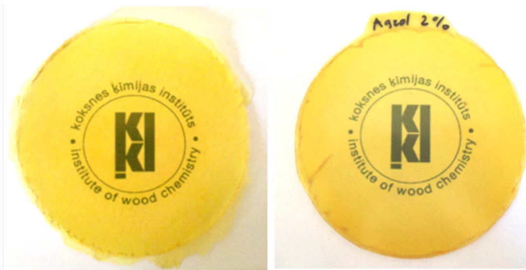
FIG. 1. Images of composites with different concentrations of CNC, 1 wt% (left) and 2 wt% (right). [Color figure can be viewed at wileyonlinelibrary.com]
