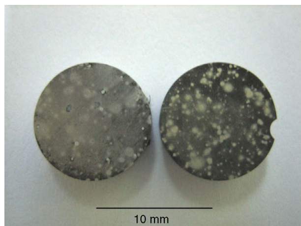
Fig. 13. Mg(PM) after 1 h–0.1 M FST (left) and 1 h–1 M FST (right) followed by 20 min immersion in PBS.
