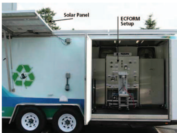
Fig. 6. DNV demonstration reactor assembled in a solar-powered trailer. Reproduced with permission from [167], N. Sridhar and D. Hill, Carbon Dioxide Utilization, Electrochemical Conversion of CO 2 —Opportunities and Challenges (2011), Position Paper 07, © 2011, Det Norske Veritas.
