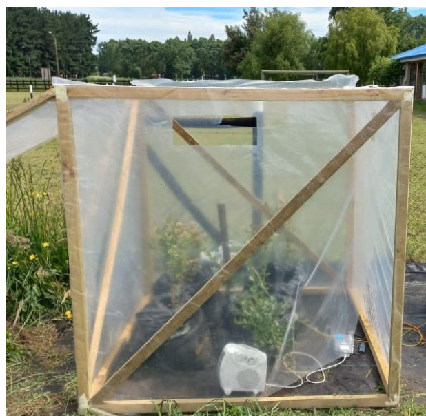
Figure 7. High-temperature chamber covered with transparent polyethylene (100 \mu\text{m} thick).
