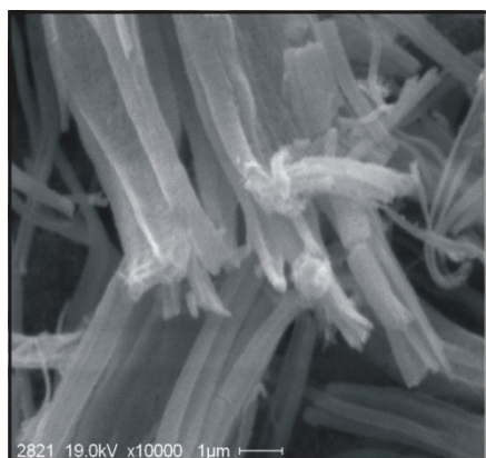
Fig. 5. Parallel ordering of faceted nanotubes (SEM).
